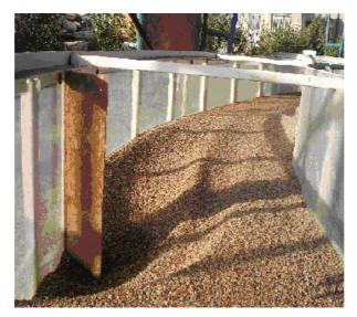
Fig. 2. Scoring and sedimatation in Spur dike downstream
